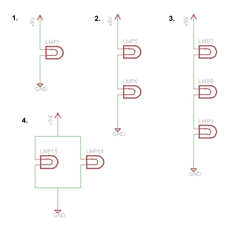
For each of these diagrams, label the relative brightness of each bulb. Use a scale of 1 to 5, with 1 being brightest, and 5 being dimmest. To get you started, the bulb in diagram #1 will have a brightness of "1". If you aren't sure with any of these, build it on your board and see how it behaves!
